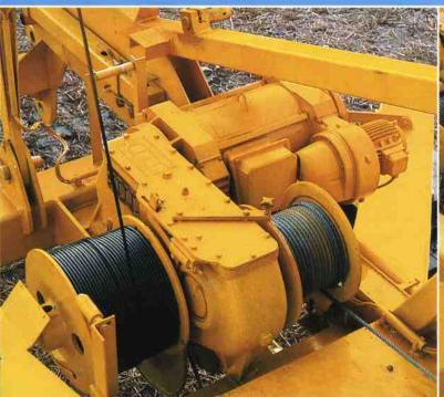
The cranes are equipped with a twin-drum winch assembly driven by a three-speed pole-changing hoisting motor; this motor has forced ventilation as well as the usual fan impeller. Forced ventilation and all-pole motor protection are reliable means of protecting against breakdowns during operation. Changeover from the hoisting to the erecting winch drum is quickly accomplished at an easily accessible drive pin.
