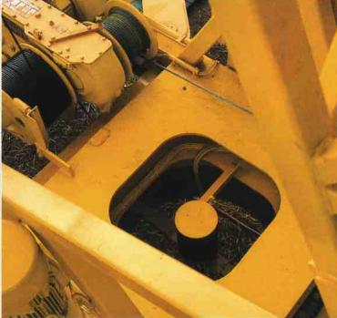
A current collector is installed between the undercarriage and the slewing platform. The advantages: unrestricted slewing in either direction, and provision for attaching the control cable to the undercarriage if desired.
