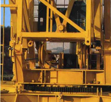
The erecting pulley block is then connected by a threaded stub shaft to the lowest tower section. Telescopic extension takes place – and the crane is ready to operate again at the new height under the hook.
