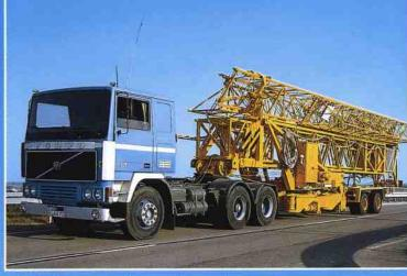
Only the semi-trailer version needs a tandem rear axle; as a trailer, single axles are sufficient.
