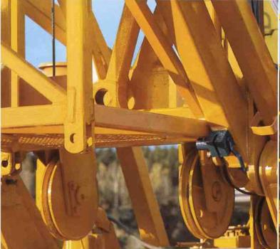
To retract a telescopic section, the erecting pulley block is simply attached to the final section of the tower, and the tower set down on the support device.
