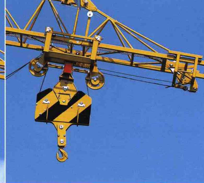
After the jib head assembly has locked itself at the jib tip, the trolley runs back and the trolley travel rope is electrically tensioned.
