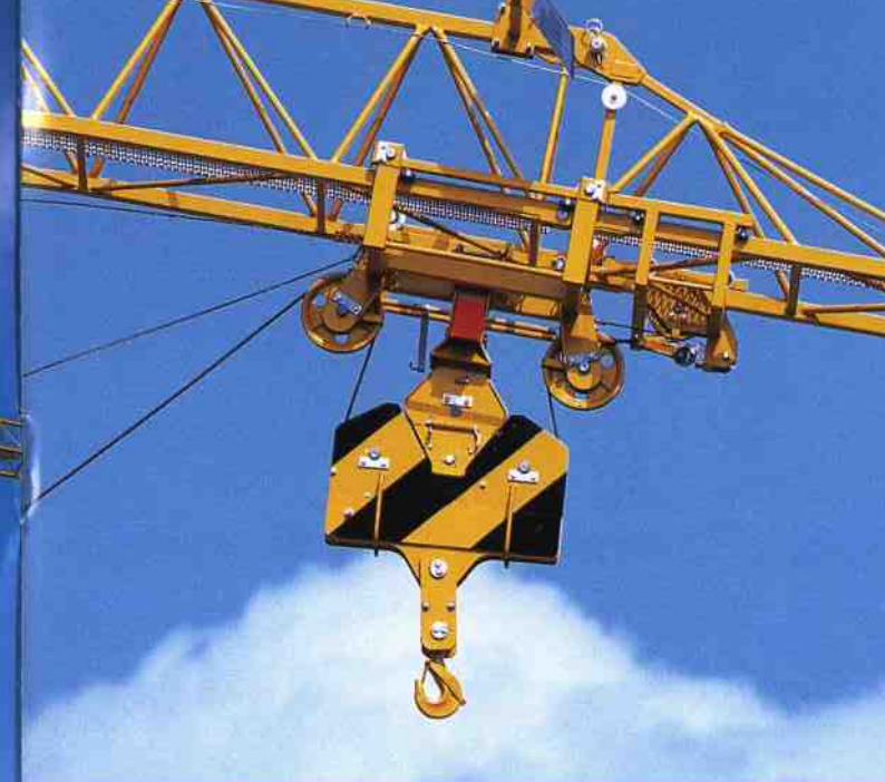
The trolley travels out the jib head assembly to the jib tip.
