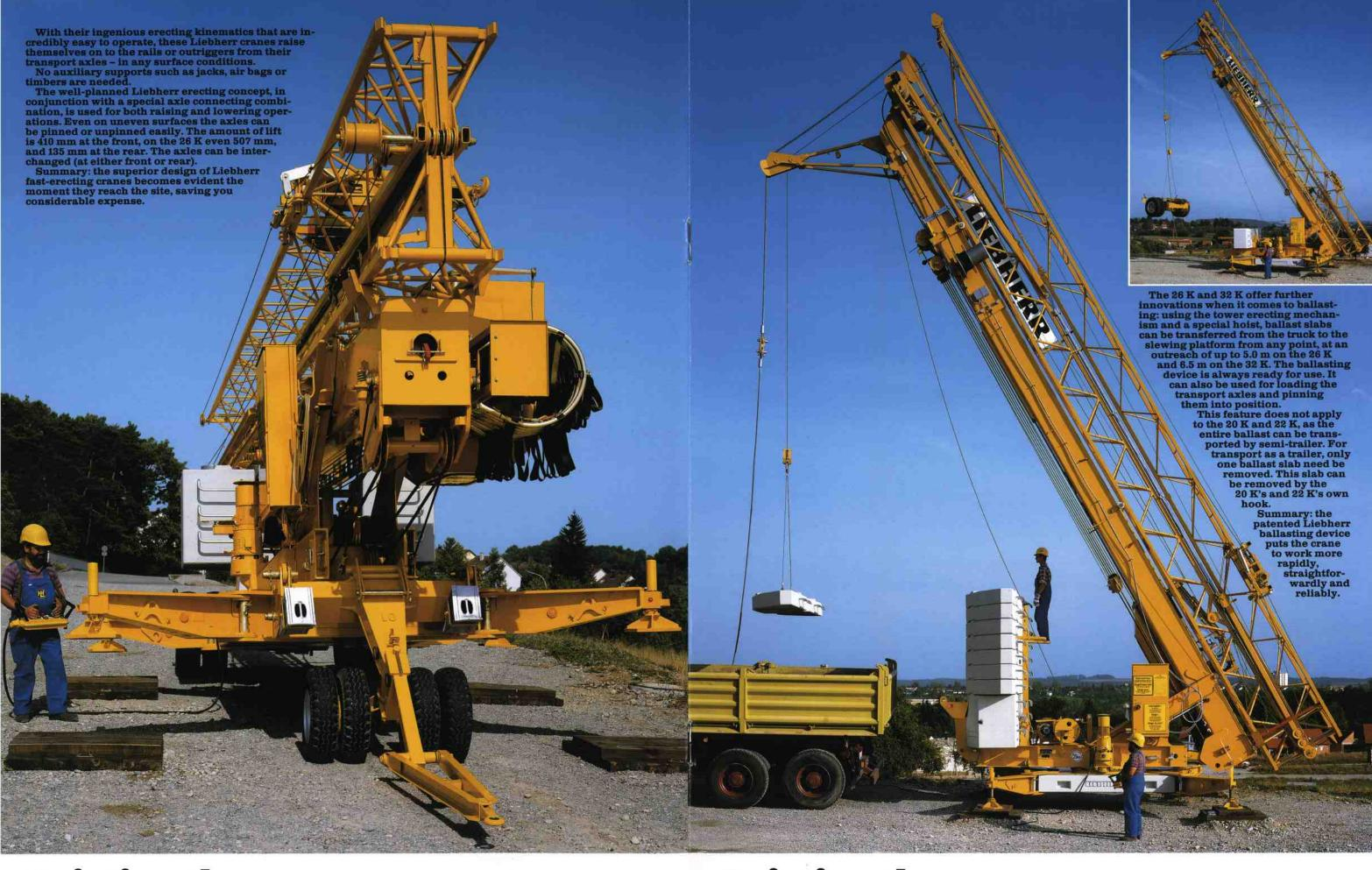
Pointing the way: mounting on outriggers or rails.
